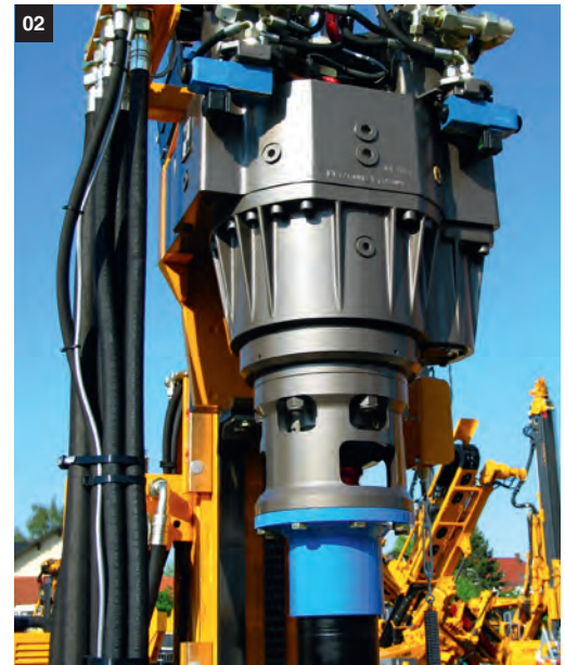
07 HDI-Ausrüstungen // Jet grouting equipment
